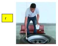
Insert demounting lever between bead and wheel disc rim. Make sure that lever is inserted properly and push the long edge of the tool down so that the bead comes out slowly. (Fig. s)
