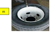
Bead seating:- In order to make sure that the bead is evenly seated on the rim, the best practice of inflating tyre assembly is in horizontal position. Place the assembled tyre rim on fitment stand. Placing the fitment stand under the wheel disc helps us to expand the tyre in a right seating area. 1 inch Height of Tyre stand shall be used keep the tyre above the ground. (Fig. n)
