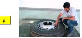
With the tyre assembly laying flat, break the bead seat of both beads with a bead breaking tool. Do not use hammers of any type to break the bead. Striking a wheel assembly with a hammer of any type can damage the tyre or wheel disc. (Fig. q)
